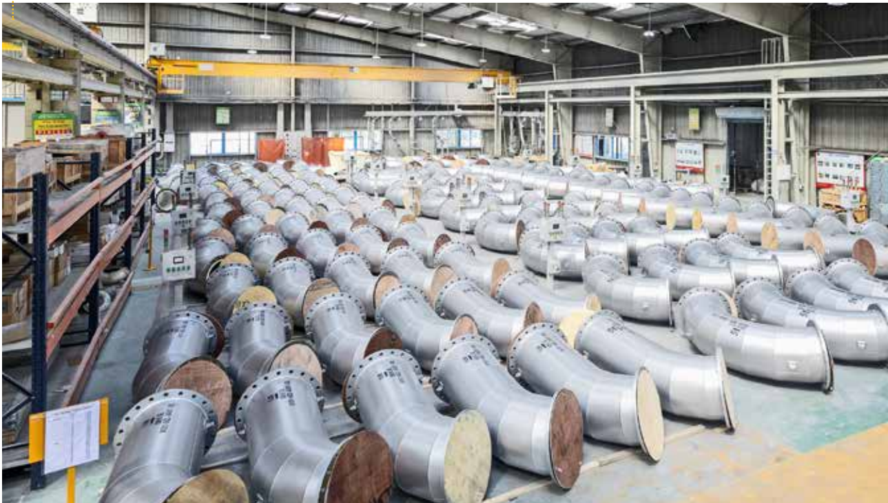
Ceramic lined steel cyclones for mineral processing industries
