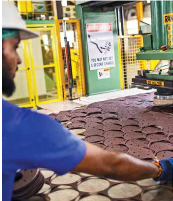
Abrasive discs used for metal, wood and composite applications being punched out at CUMI's Sriperumbudur facility
