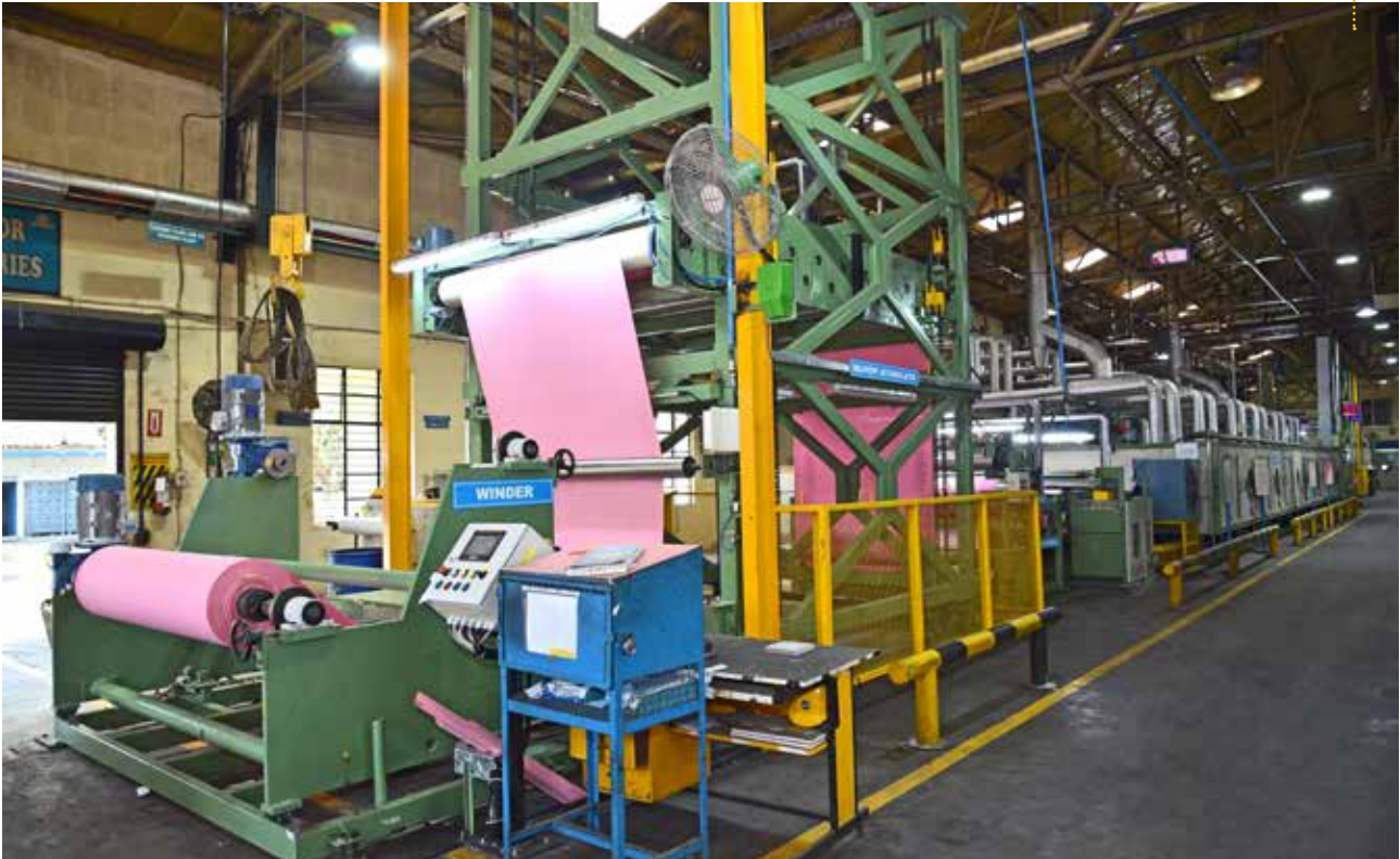
Stenter at Maraimalai Nagar, processes cloth backings for Coated Abrasives
