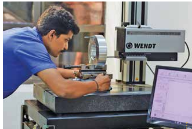
Precision measurement of contours in a CMM machine
