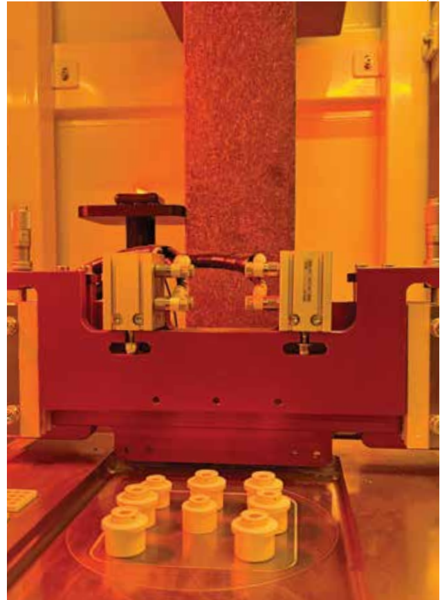
3D printer from 3DCeram to manufacture complex ceramic parts
