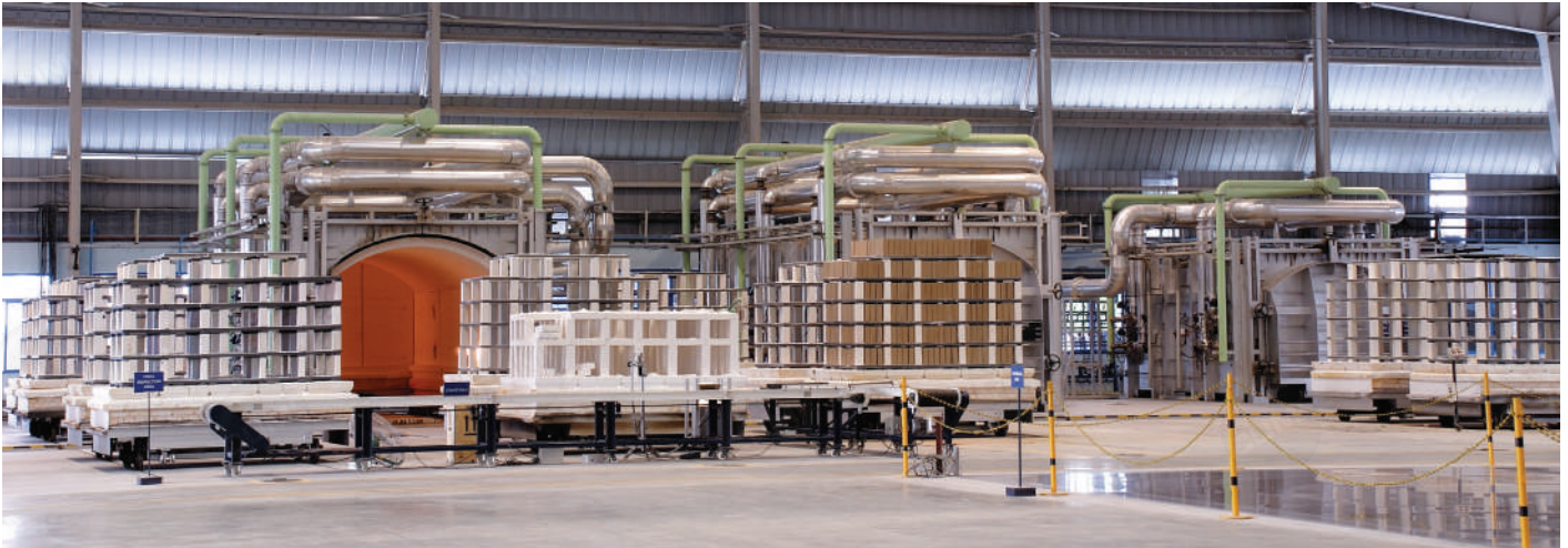
Batch Kilns with operating Temp. upto 1750°C
